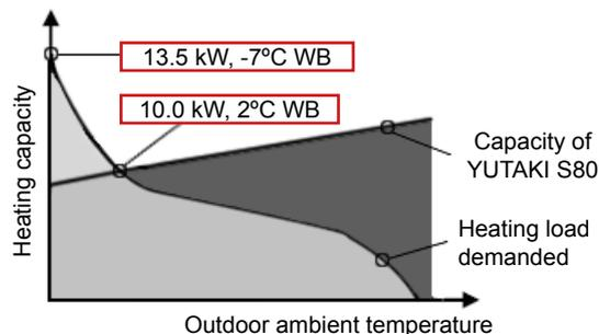
In this new system, the heat pump meets the regular heating load. The electric heater can provide the auxiliary heating capacity required to cover the peak heating load of 13.5 kW (-7 °C WB) on the coldest days of the year.
