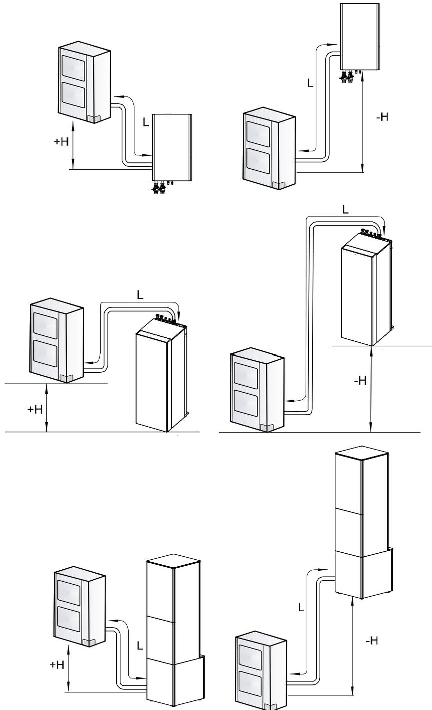
**H:** Height difference between indoor unit and outdoor unit (m).
