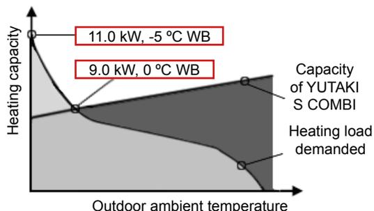
In this new system, the heat pump meets the regular heating load. The electric heater can provide the auxiliary heating capacity required to cover the peak heating load of 11.0 kW (-7 °C WB) on the coldest days of the year.
