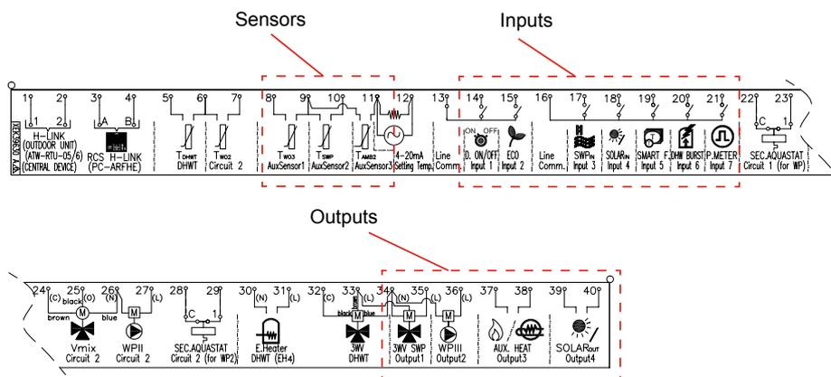
The following input, output and sensor functions can be selected through the “I/O and sensor” menu of the controller:
