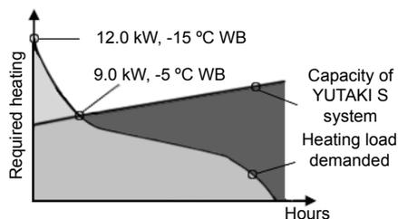
These conditions determine the position in the Maximum heating capacity tables (See section “[4.3.1 Maximum heating capacity table \(kW\) \(Integrated\)](#)”, where it can be confirmed whether the unit has enough heating capacity to cover the regular heating load required by the installation (9.0 kW for an inlet/outlet water temperature of 30/35 °C and an ambient temperature of -7 °C WB).
