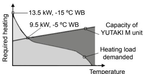
These conditions determine the position in the table of “4.6.1 Maximum heating capacity table (kW) (Integrated)” section, where it can be confirmed whether the unit has enough heating capacity to cover the regular heating load required by the installation (10.5 kW for an inlet/outlet water temperature of 40/45 °C and an ambient temperature of -7°C WB).
