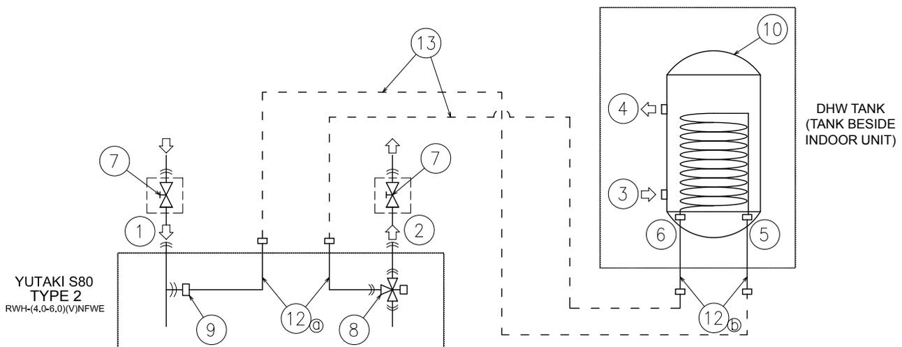
When installing the YUTAKI S80 indoor unit TYPE 2 (RWH-(4.0-6.0)(V)NFWWE) in combination with the HITACHI DHW tank (DHWS(200/260)S-2.7H2E) the following elements to provide DHW operation are needed:
