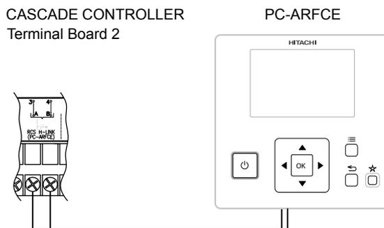
For this purpose, a H-LINK cable (accessory) is necessary.
