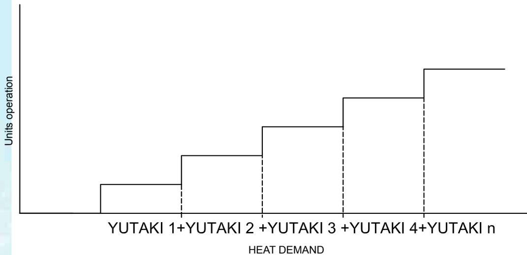
When this control determines that a unit has to be switched ON or OFF, it is the rotary token control which determines the concrete unit to be switched ON or OFF.
