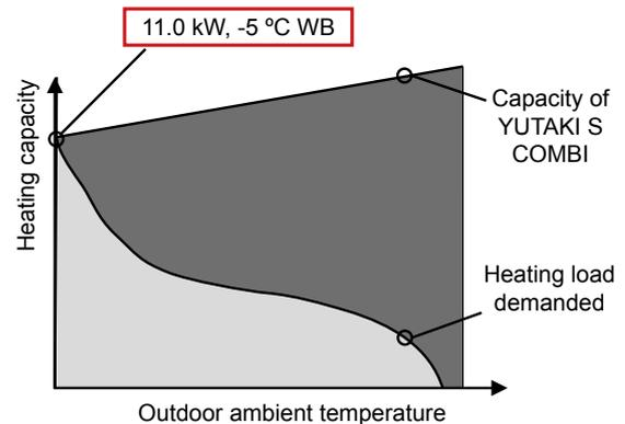
These conditions determine the position in the Maximum heating capacity tables (see section “4.4.1 Maximum heating capacity table (kW) (Integrated)”, where it can be confirmed whether the unit has enough heating capacity to cover the heating load required by the installation on the coldest day of the year (11.0 kW for an inlet/outlet water temperature of 30/35 °C and an ambient temperature of -2 °C WB).
