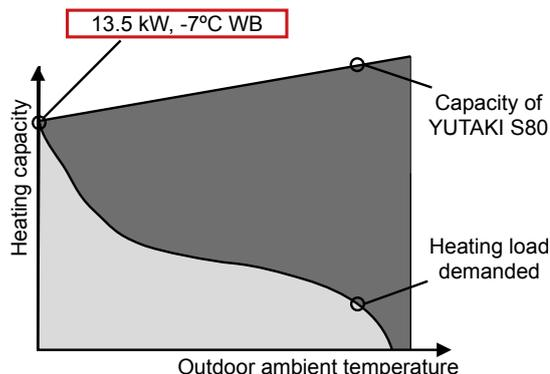
These conditions determine the position in the Maximum heating capacity tables (see section “4.5.1 Maximum heating capacity table (kW) (Integrated)”), where it can be confirmed whether the unit has enough heating capacity to cover the heating load required by the installation on the coldest day of the year (13.5 kW for an inlet/outlet water temperature of 47/55 °C and an ambient temperature of -7 °C WB).
