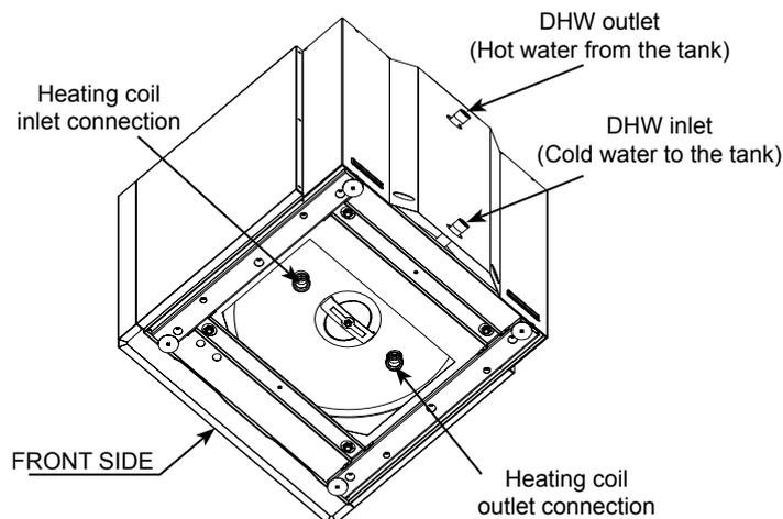
**Heating coil pipes (Factory-supplied with the DHW tank accessory (DHWS(200/260)S-2.7H2E(-W)))**
