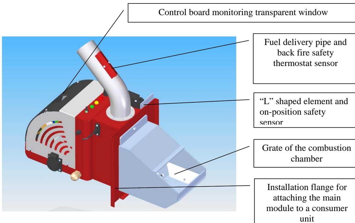
**Figure 3.3** Side view of the main unit of the burner;
