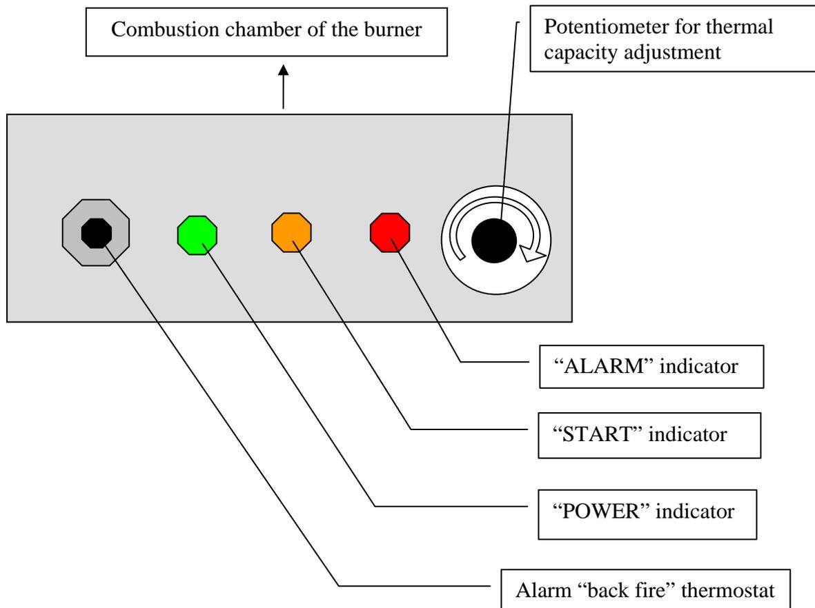
**Figure 5.1.** Interface board, equipped with indicator lamps, control and safety elements of automatic pellet burner “ERATO GP20+”.
