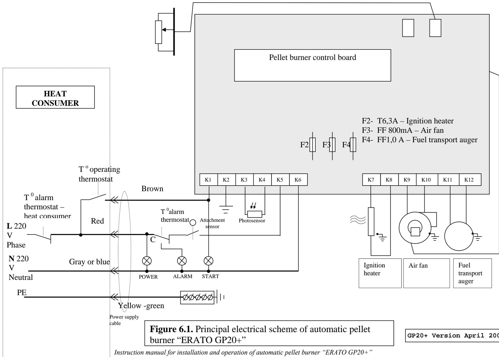
**Figure 6.1.** Principal electrical scheme of automatic pellet burner “ERATO GP20+”
