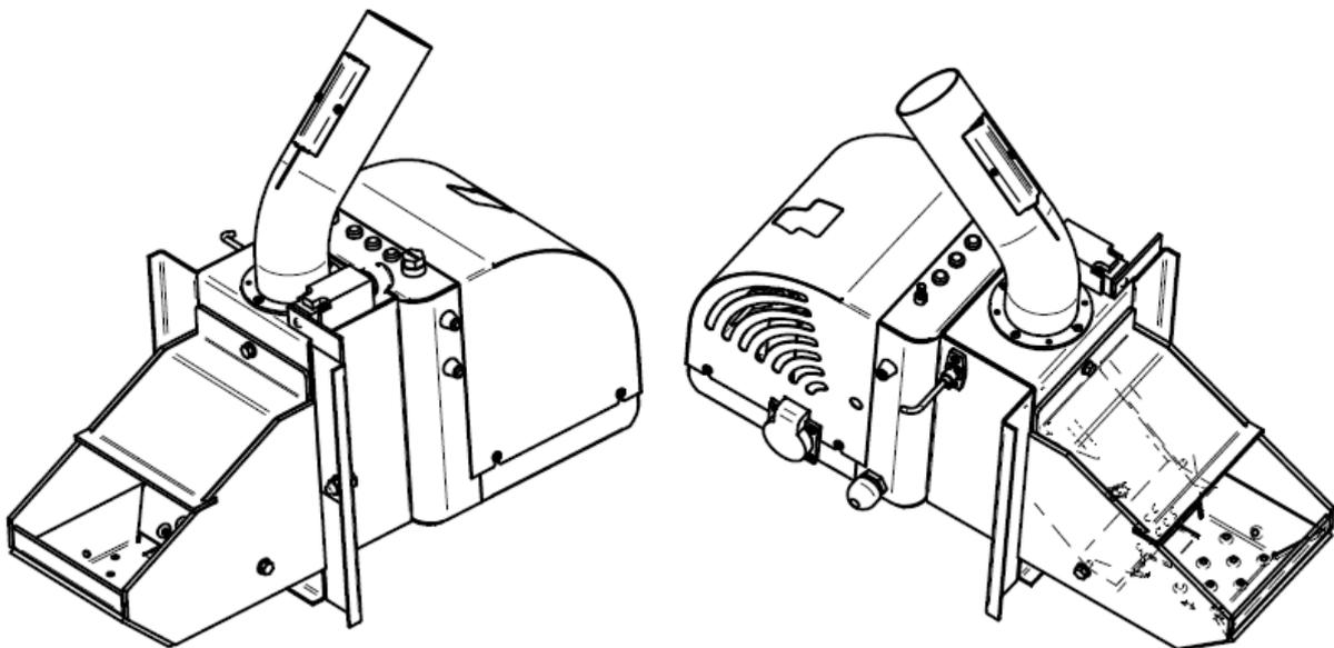
**Figure 4.1.** Isometric view of the main unit of the burner – *side view*;
