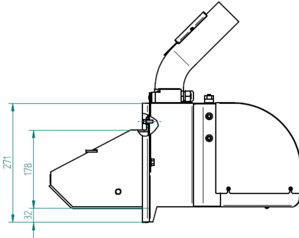
**Figure 4.2.** Overall and characteristic dimensions of the main unit – *side view*;
