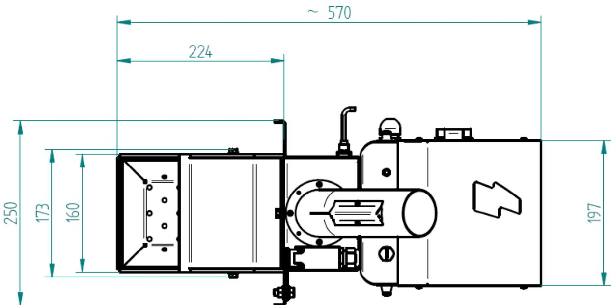
**Figure 4.3.** Overall and characteristic dimensions of the main unit – *top view*;
