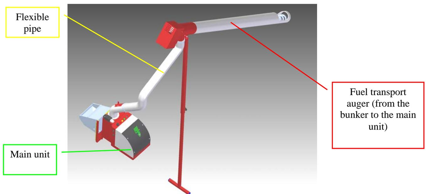
**Figure 3.1** Arrangement of the modules of the pellet burner (*top view*);
