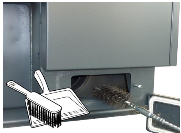
Sample cleaning and ash removing from the bottom part of the flue way - bottom lid
