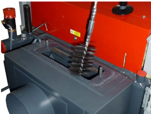
Sample cleaning of the flue way with a wire brush - upper lid
